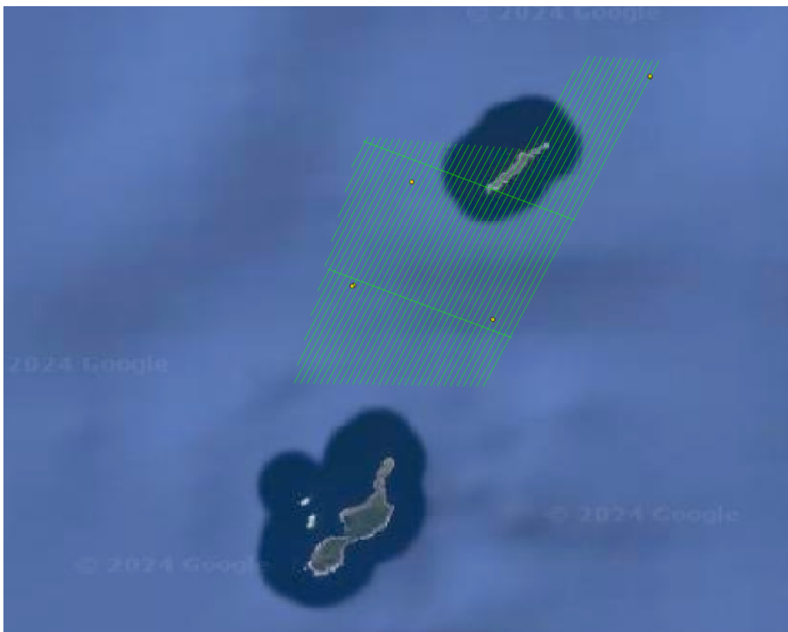
Figure 5 Area and flight lines for aerial magnetometer survey August 2024 (Thomson Airborne, Google Earth).
