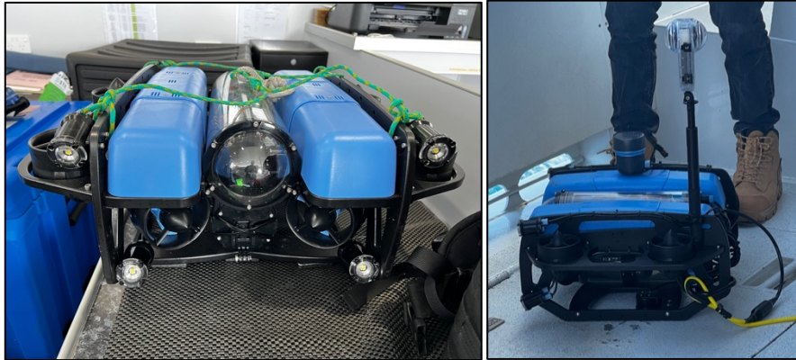
Figure 11 BlueROV used to record site. Image on right shows Insta360 camera mounted for data capture (WA Museum).
