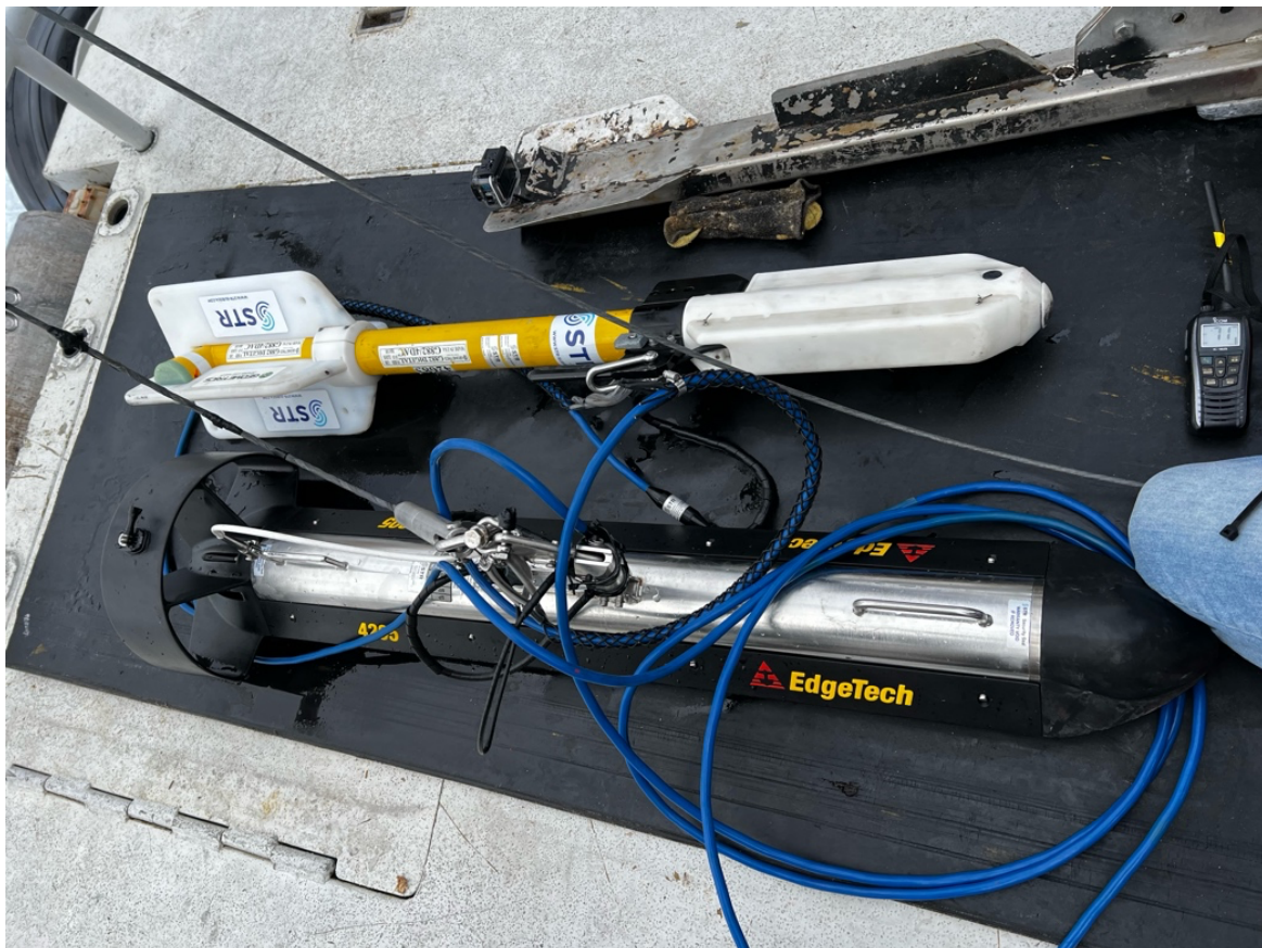
Figure 7 EdgeTech 4205 side scan sonar and Geometrics G-882 magnetometer (WA Museum).
